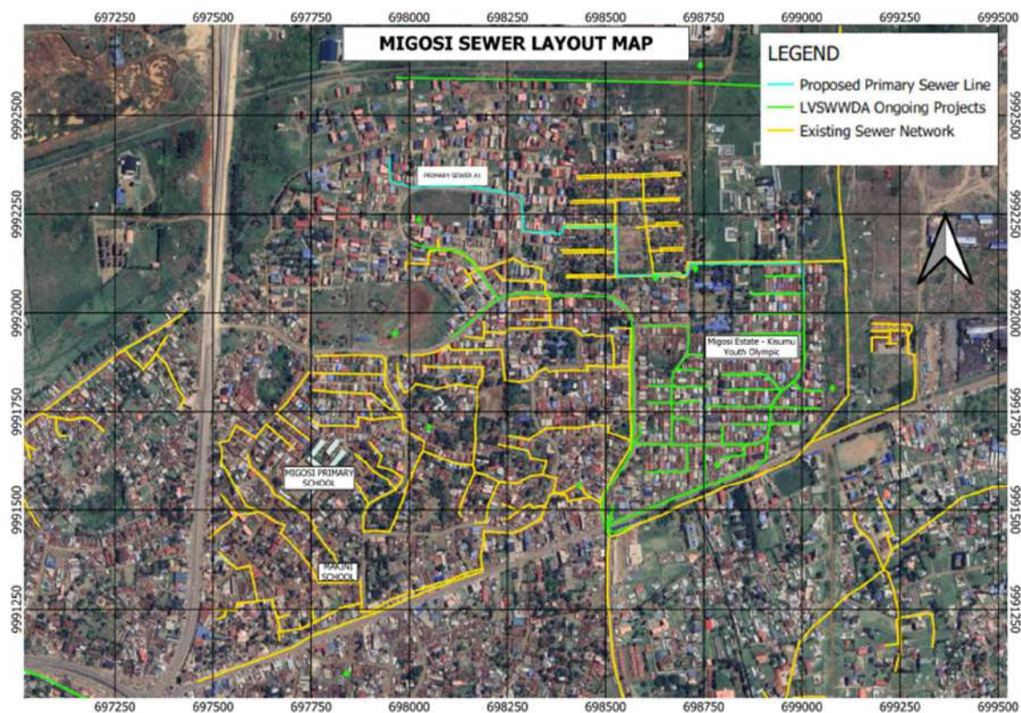
Figure 2.21: Migosi proposed sewer design layout plan
