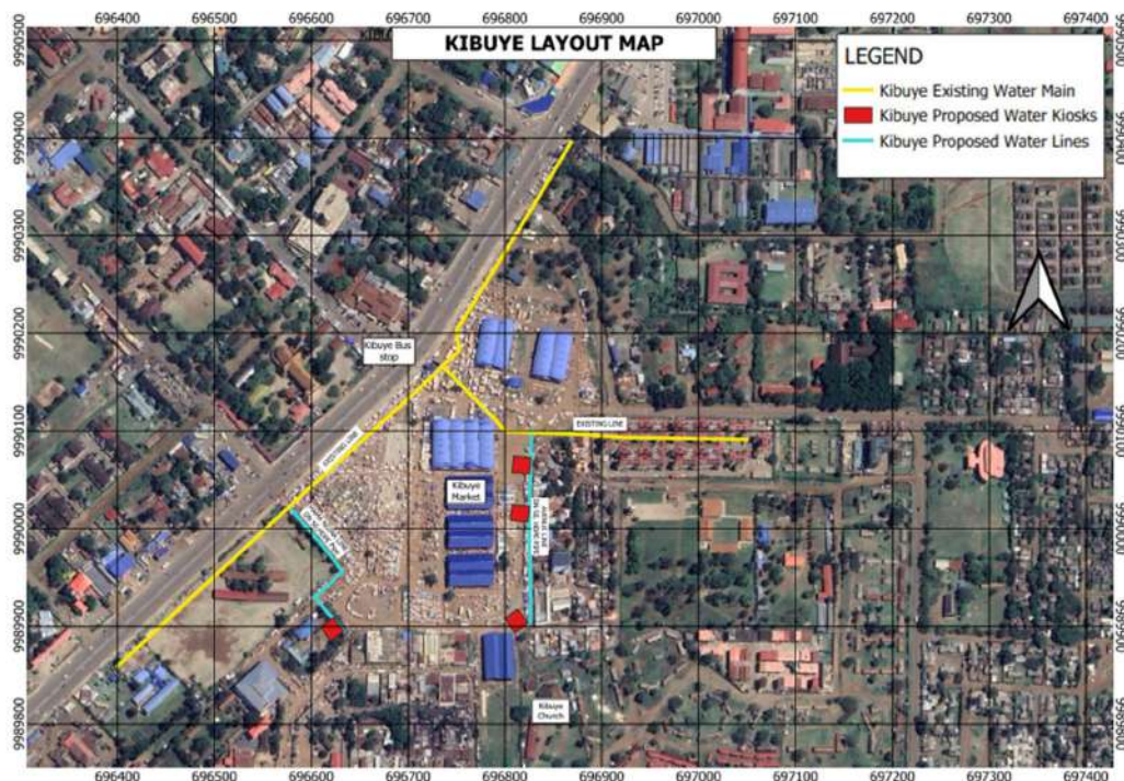
Figure 2.17: Kibuye proposed water supply layout plan
