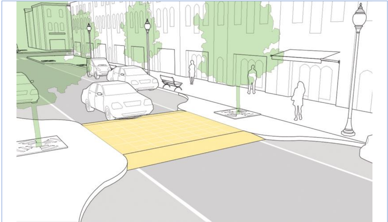
Figure 2-5: Typical Speed Bump Crosswalk
